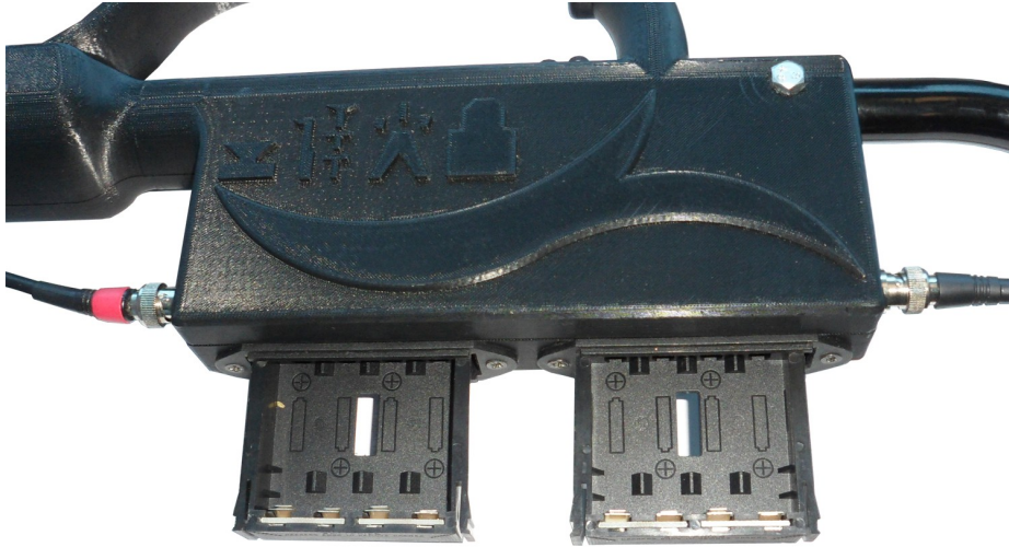
Illustration 5.1: Main Unit with extended battery housings.
