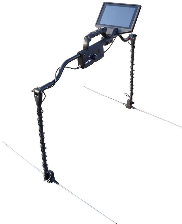
Illustration 5.8: Fully assembled Gepard - GPR unit
